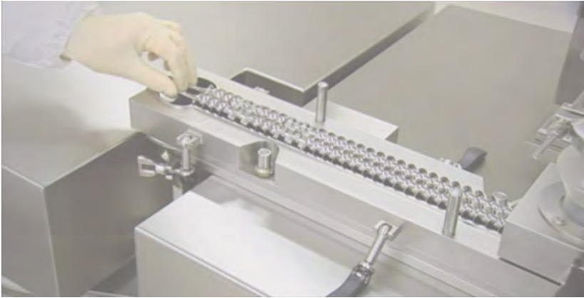
Figure 3.4: Twin-screw granulator from lab-scale continuous processing equipment ConsiGma TM -1 with the granulator barrel that can be opened.
